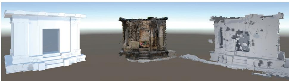
Figure 1. From left to right: manual reconstruction, point cloud, automated voxel reconstruction. (Source: authors).
