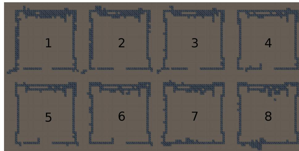
Figure 2. Temple split into voxel slices. Here we have a selection of slices from the centre part of the above temple, numbered 1-8 from top to bottom. This clearly shows the door and structure of the temple, abstracting away some of the noisiness of the point cloud and allowing us to focus on the overarching geometric elements. (Source: authors).
